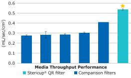
Comparison of media flow rate among multiple vacuum-driven filters. 500 mL of DMEM with 10% FBS was filtered through various sterile filter cup devices and timed.
