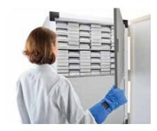
Figure 2. Adaptive control of cooling. The V-drive technology featured in TSX Series freezers is designed to detect conditions such as multiple door openings and adjust to a higher compressor speed when required.
