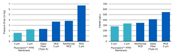
Lower pressure drop, lower FWHM\* measurements. Our Fluoropore<sup>™</sup> PTFE membranes exhibit lower pressure drop (A) and collect particles on the surface, providing better detection efficiencies and lower FWHM measurements (B). Room air was collected at 1.7 m<sup>3</sup>/h (1 standard cubic foot/min).
