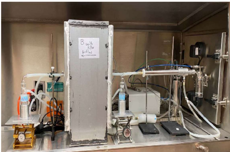
Figure 1A (Left). Laboratory hood set up with aerosolization and detection equipment and the Genesis Air unit housing the MERV 13 filter. From right to left: nebulizer, an upstream Biosampler, MERV 13 filter, Genesis Air unit housing filter, and a downstream Biosampler. Figure 1B (Right) A schematic diagram of the experimental set up showing the pathway of the aerosolized virus from right to left as traveling out of the nebulizer, through upstream Biosampler, though the filter housed in the inactive Genesis Air unit, and finally back through a downstream Biosampler.
